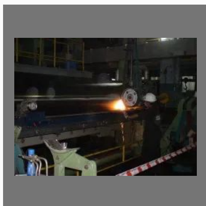
Grinding On Rope Reel
