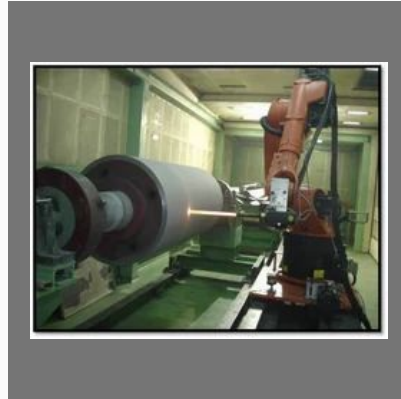
TWAS Coating On Boiler Tube
