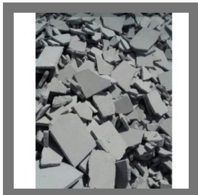
Broken AAC Block
