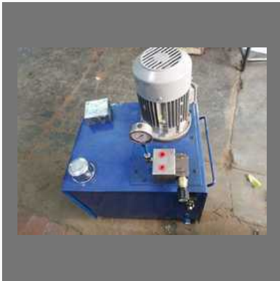
Hydraulic Power Pack
