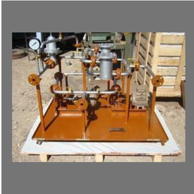
Duplex Pumping Unit
