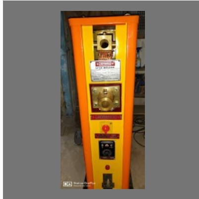
Spot Welding Machine
