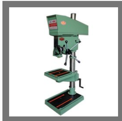
Heavy Drilling Machine
