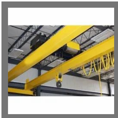
Double Girder Overhead Traveling Cranes
