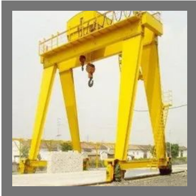
Electric Gantry Crane
