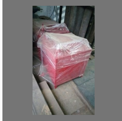
Diesel Storage Tank
