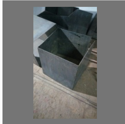
MS Diesel Storage Tank
