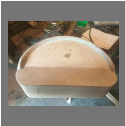
Truck Speedometer Wooden Pattern
