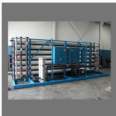
Reverse Osmosis Equipment
