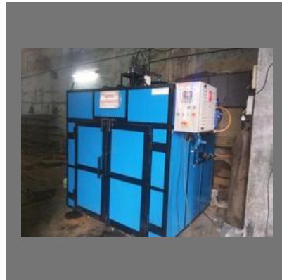
Powder Coating Electrical Oven
