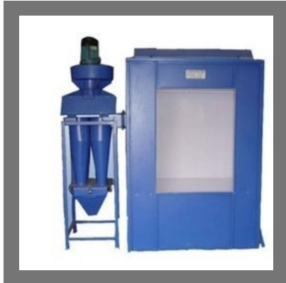
Powder Coating Spray Booth
