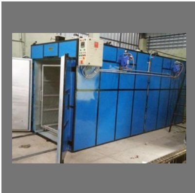
Powder Coating Gas Fired Oven
