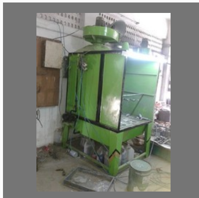
Painting Booth with Water Curtain Tank
