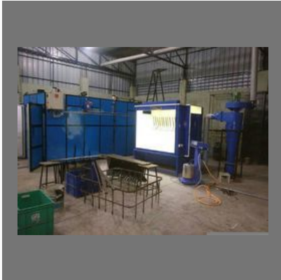
Powder Coating Spray Booth
