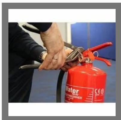
Fire Extinguisher Refilling
