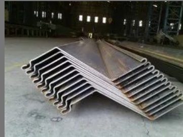
Sheet Piling Shoring
