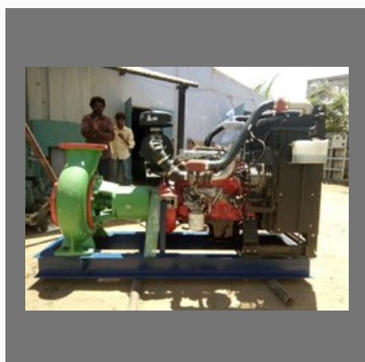
Diesel Engine Driven Dewatering Pump
