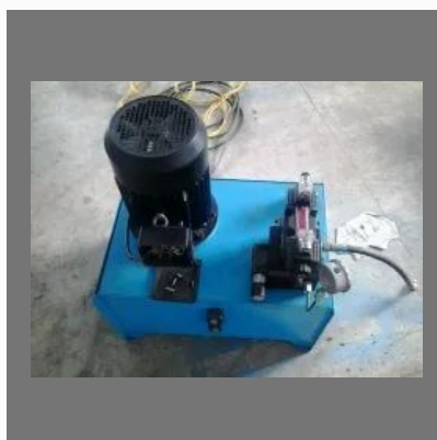
Hydraulic Power Pack
