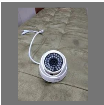
Dome CCTV Camera
