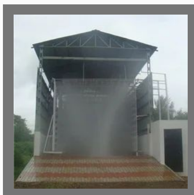
Drive-In Rain Test Chamber Twin Shower
