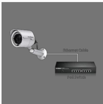
Network Camera Installation
