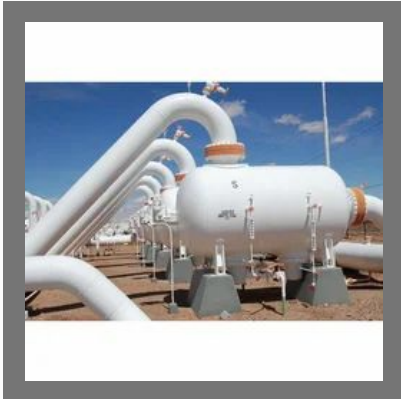
Industrial Gas Scrubber
