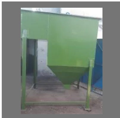
Fabricated 30KLD MS FRP Coated ETP
