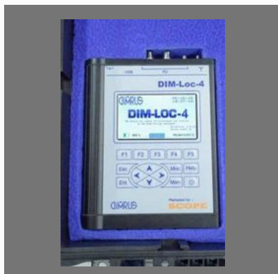
Portable Partial Discharge Monitor
