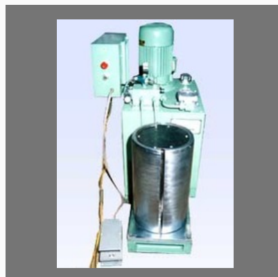
Drum Expander Machine for 20 ltr. & 25 ltr. Drum
