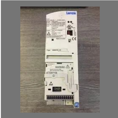
Lenze VFD For Boiler
