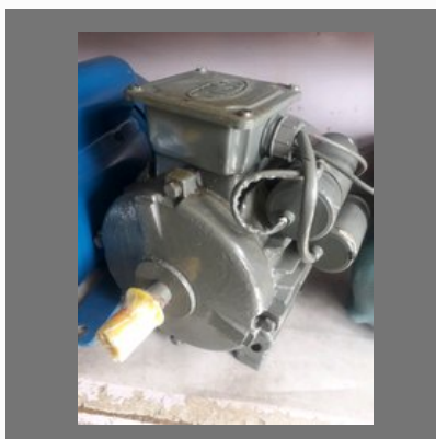
Water Pump Motor
