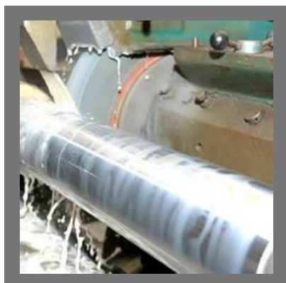
Grinding Job Work
