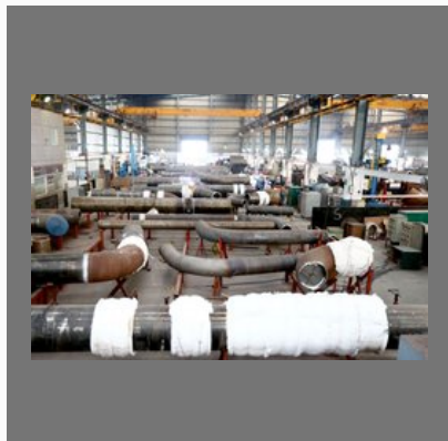
Shop Fabricated Pipe Spools
