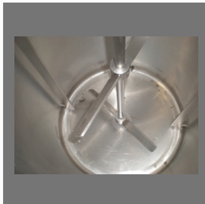
SS Mixing Tank
