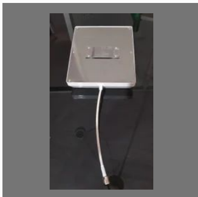
Patch Panel Antenna
