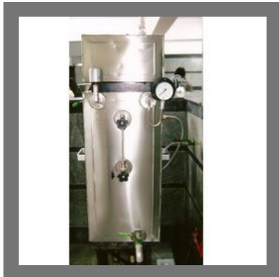
SS Steam Boiler
