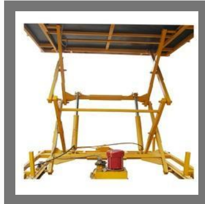
Material Loading Unloading Lift
