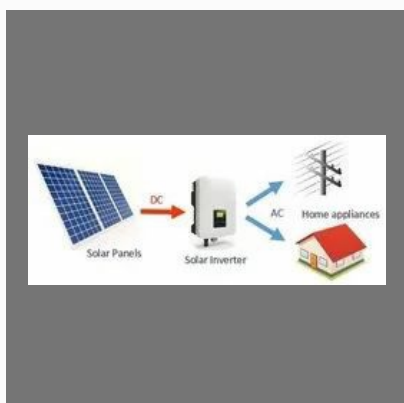
Solar On Grid Power Plant
