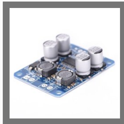
TPA3118 PBTL Mono Digital Amplifier Board 1X60W 12V 24V Power Amplifier AMP
