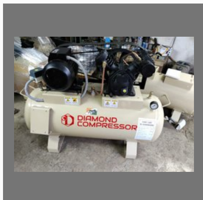
Two Stage Air Compressor
