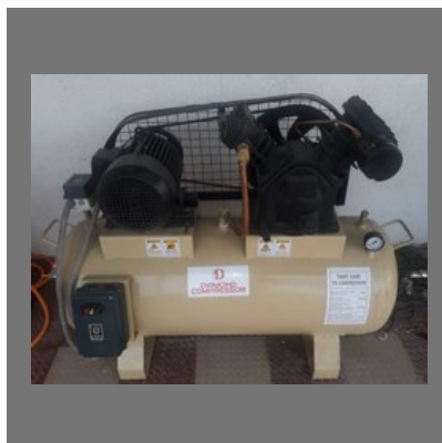
Two Stage Air Compressor
