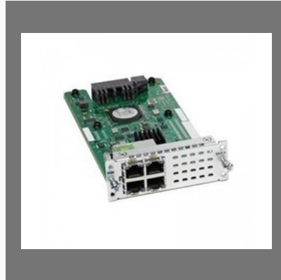
Cisco 4-Port Gigabit Ethernet Switch NIM (NIM-ES2-4)
