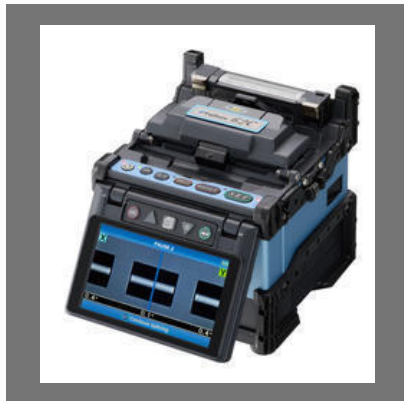
Traditional Core Alignment Fusion Splicing Machine
