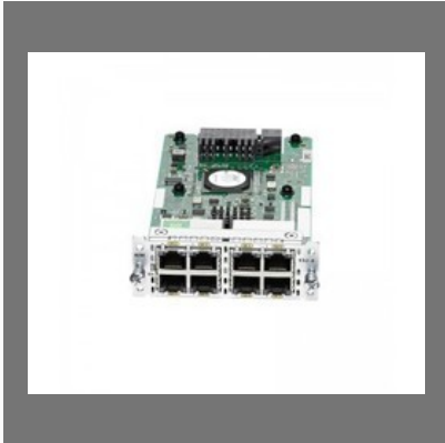
Cisco 8-Port Gigabit Ethernet Switch NIM (NIM-ES2-8)
