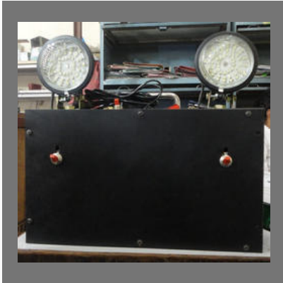
Emergency Exit Light
