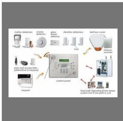
Burglar Alarm System
