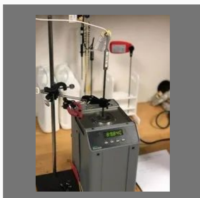
Temperature Gauge Calibration
