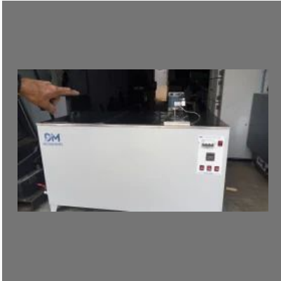
MS Curing Tank
