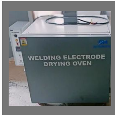
Welding Electrode Drying Oven
