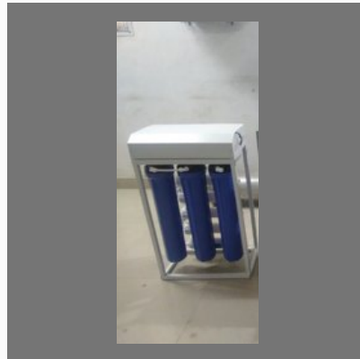
50LPH RO Plant
