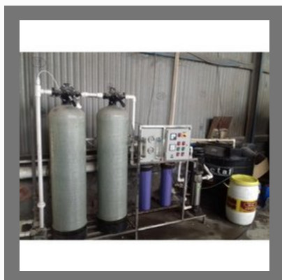
500 LPH FRP RO Plant
