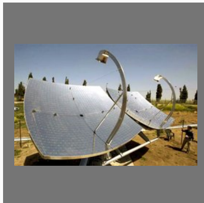
Parabolic Solar Dryer
