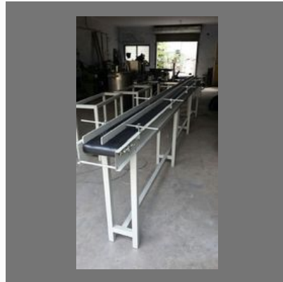
MS Belt Conveyor with VFD
