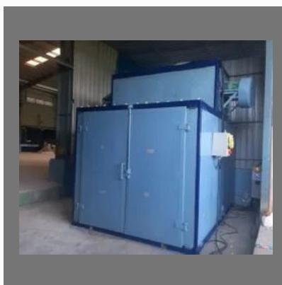
Paint Curing Ovens
