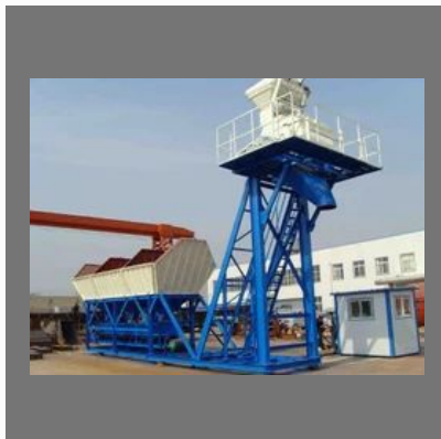
Automatic Batching Plant
