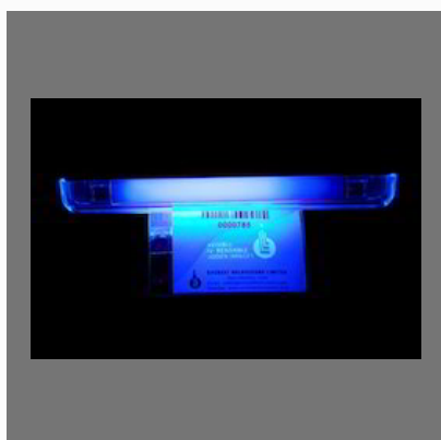
Holographic Integrated UV Readable Image and Text Label
