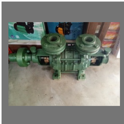
Boiler Feeding Pump
