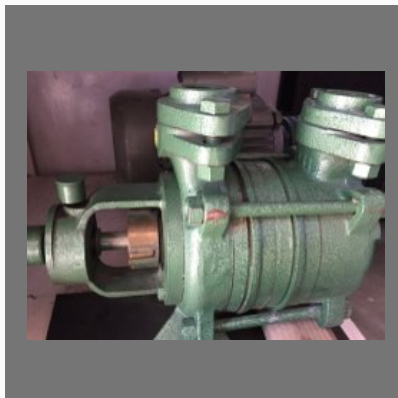
Boiler Feeding Pump
