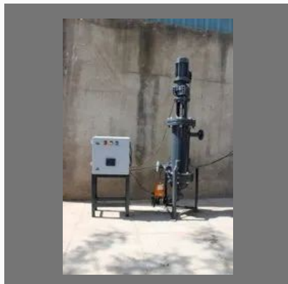
Self Cleaning Filter
