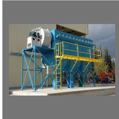
Centralized Dust Collection System
