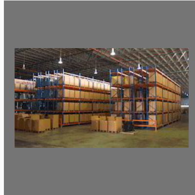
Double Deep Pallet Racks
