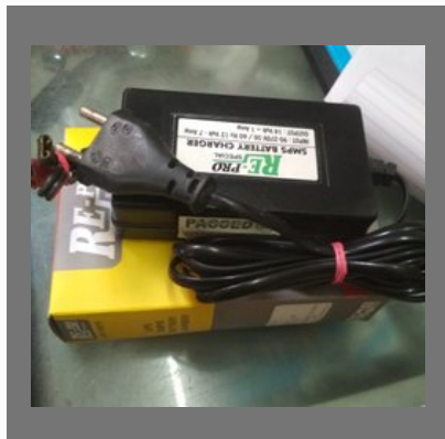
SMPS Battery Charger
