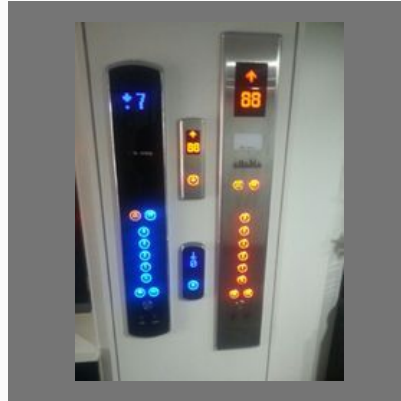
Car Operating Panel
