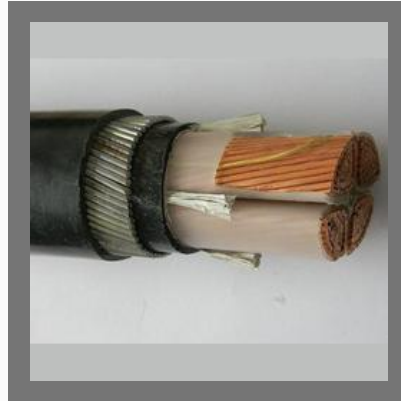
Four Core Cable CU PVC PVC SWA PVC Power Cable 600 to 1000 V
